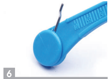
6 Check that the key has reached the stop on the circular end of the handle.
