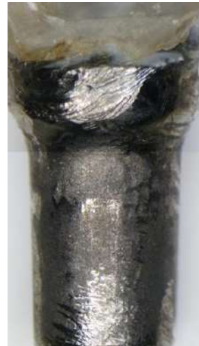
Examples of abutments with damaged or altered Morse taper.
