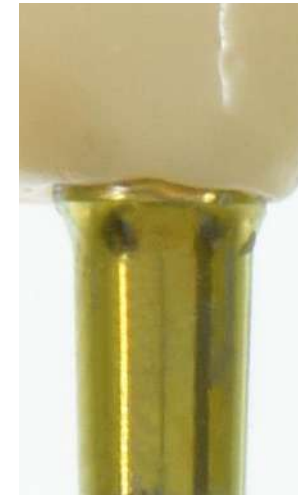
Examples of abutments with damaged or altered Morse taper.
