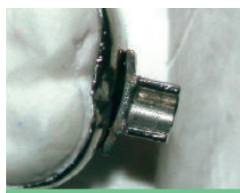
The connector's flanges ensure a good joint to the band by means of a welding machine
